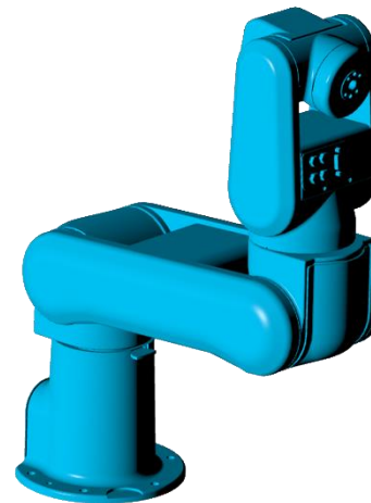
Figure 9-4: C := 3, Wrist flip, elbow below, base forward.
