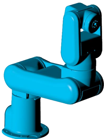
Figure 9-5: C := 4, Wrist no flip, elbow below, base backward.
