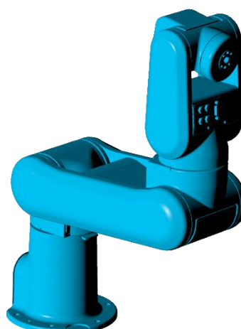
Figure 9-6: C := 5, Wrist flip, elbow below, base backward.
