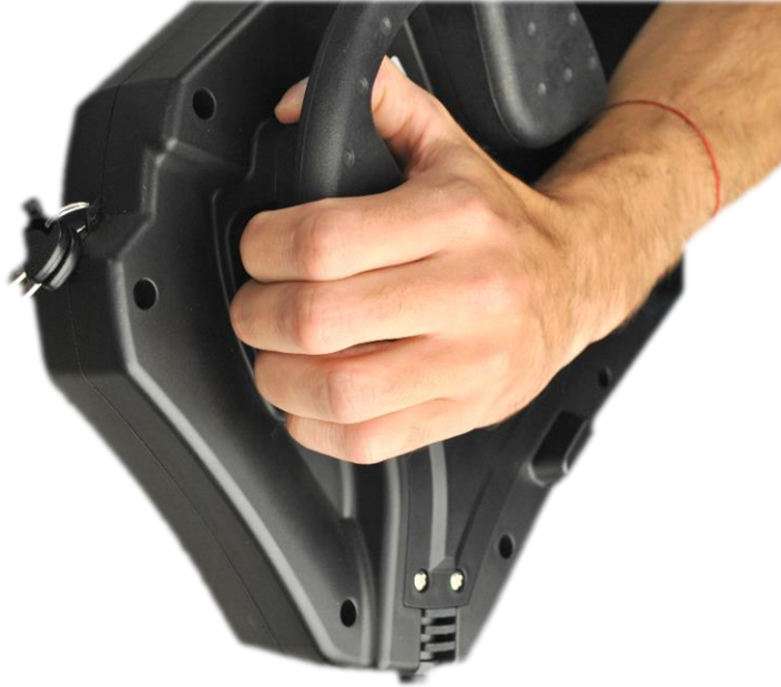
Figure 2-9: Demand switch pressed
