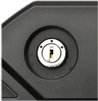
Figure 2-10: Key switch real Teach Pendant
